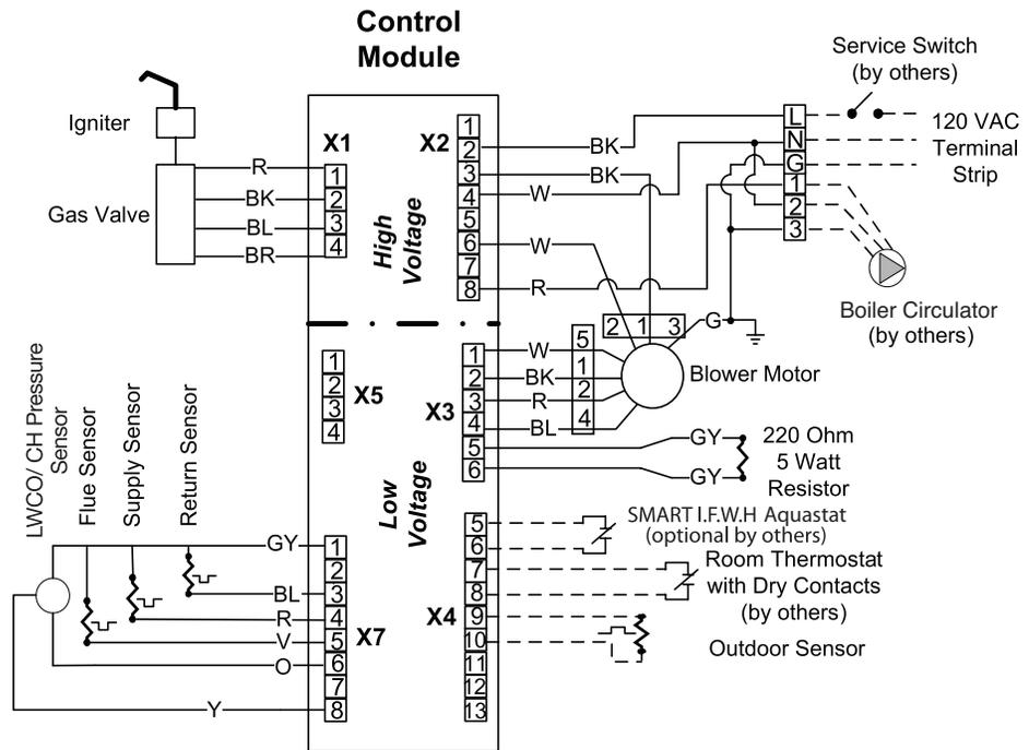
**Note** - The wiring for 120V field connections to the appliance shall have a minimum size of 14 AWG and a temperature rating of at least 194°F (90°).
