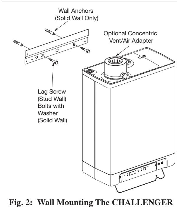
**Fig. 2: Wall Mounting The CHALLENGER**
