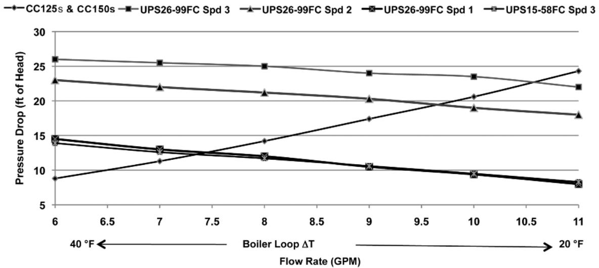
Graph 9 : Pressure Loss Through Boiler - Grundfos Circulators
