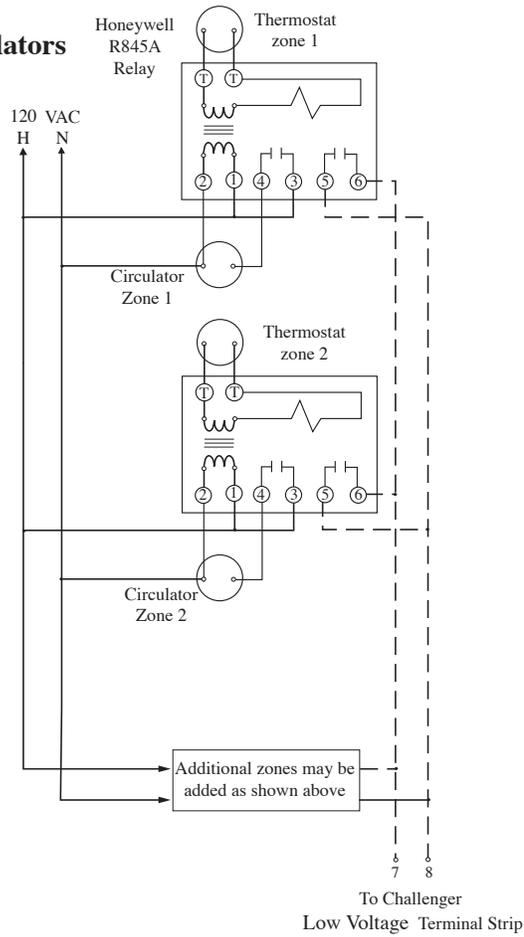
**Fig. 21: Typical Zone Relay Panel Wiring**
