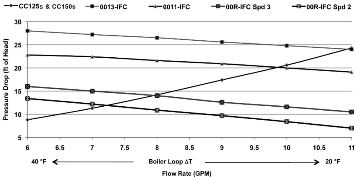
Graph 10 : Pressure Loss Through Boiler - Taco Circulators
