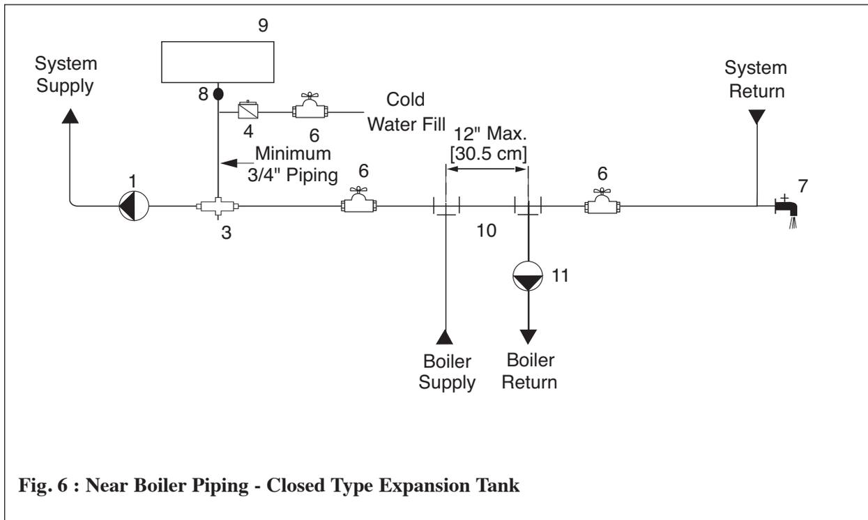
**Fig. 6 : Near Boiler Piping - Closed Type Expansion Tank**
