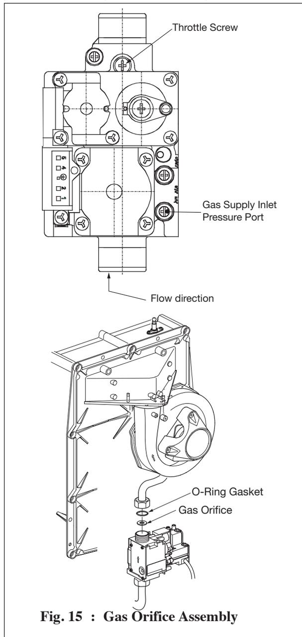
**Fig. 15 : Gas Orifice Assembly**
