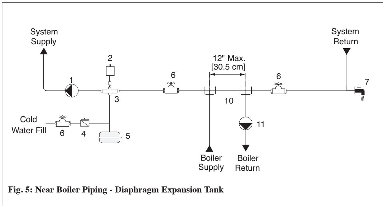
**Fig. 5: Near Boiler Piping - Diaphragm Expansion Tank**
