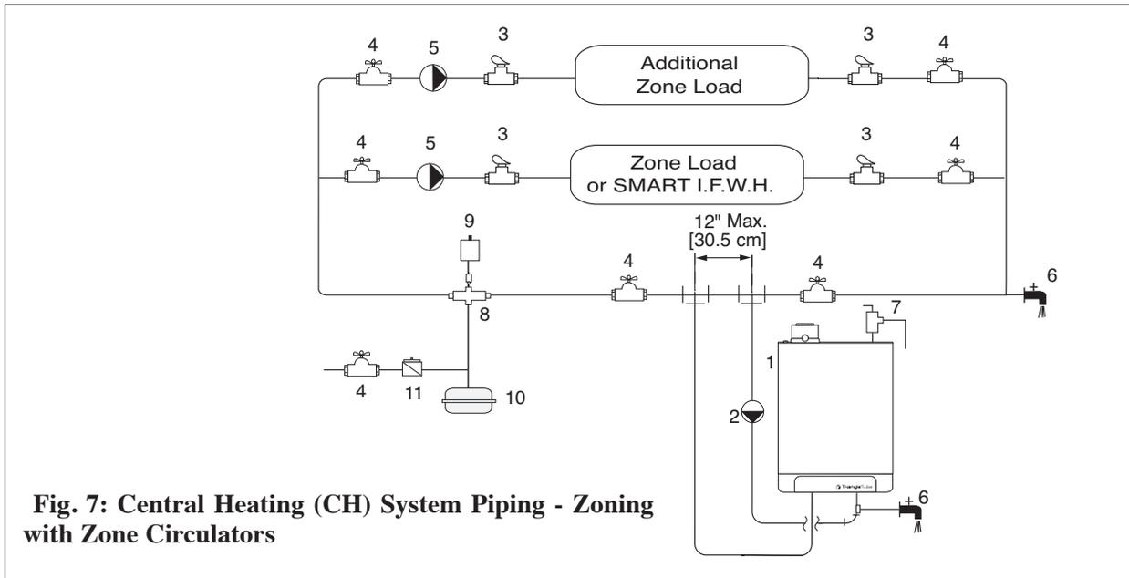
**Fig. 7: Central Heating (CH) System Piping - Zoning with Zone Circulators**
